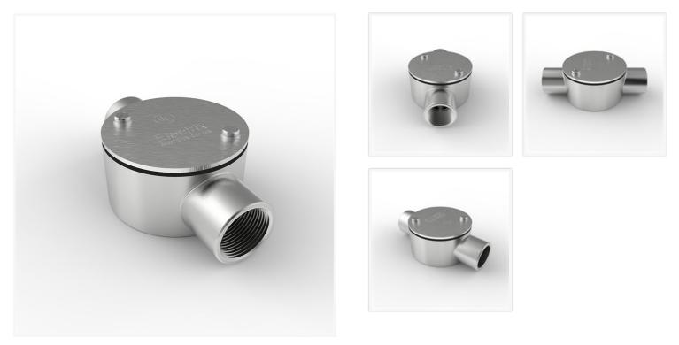
Electrix® Metric Conduit Through Boxes, in 316C16F stainless steel with a 316L - V4A - 1.4404 stainless steel lid, can be used as an inspection point and pull box during a long conduit run.
